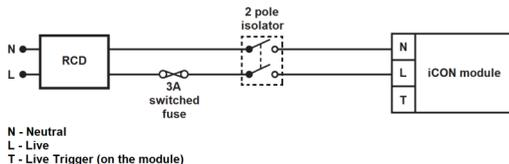
**Diagram B** - module wiring with external switching (live trigger connection used):
